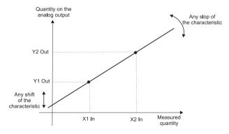
Fig. 11. Individual characteristic of analog output
