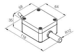
Fig. 3. Overall dimensions of the P18(D) transducer
