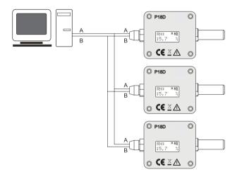
Fig. 13. Connecting the RS-485 interface.
